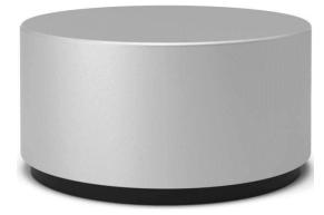
Microsoft's Surface Dial provides a way to interact physically with Windows 10 Creators Update or later, and applications that run under it. Although called the "Surface" Dial, it requires only Bluetooth; you do not need a Surface-family computer. However, the Surface 5 and Surface Studio do support using it on their touch-compatible screens, not just as a tabletop device.
